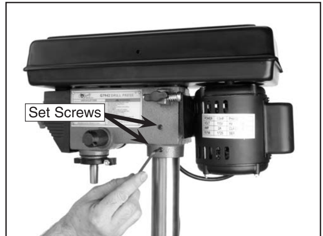
Figure 11. Securing headstock with set screws.
